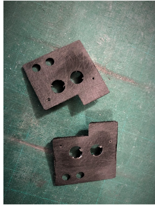
Roughen the Servo trays bottom
