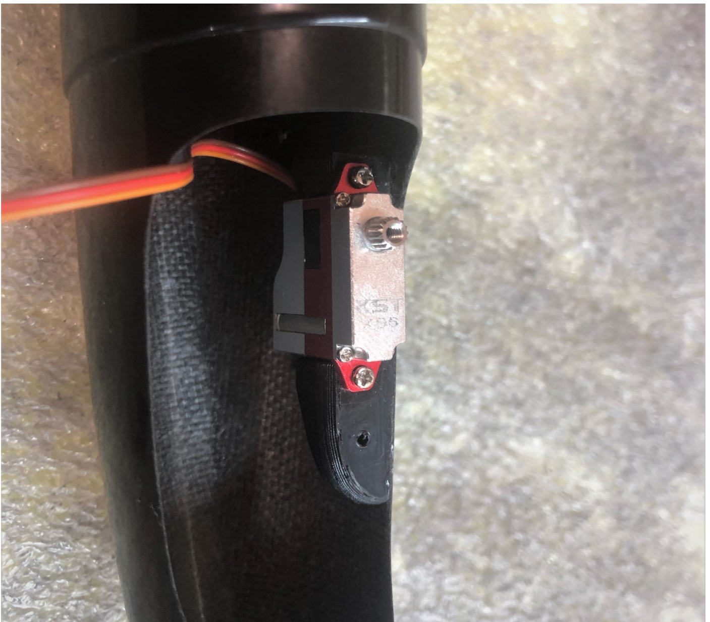
Glue with epoxy or super glue/cyanoacrylate
