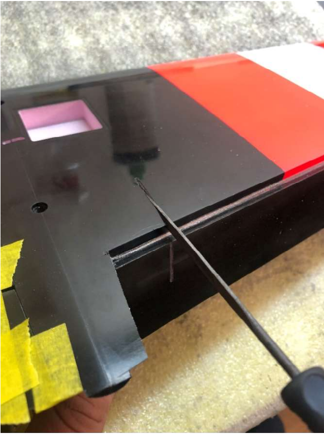
With a rectangular section jewellers file widen the slot in the foam to let the elevon linkage move freely.
