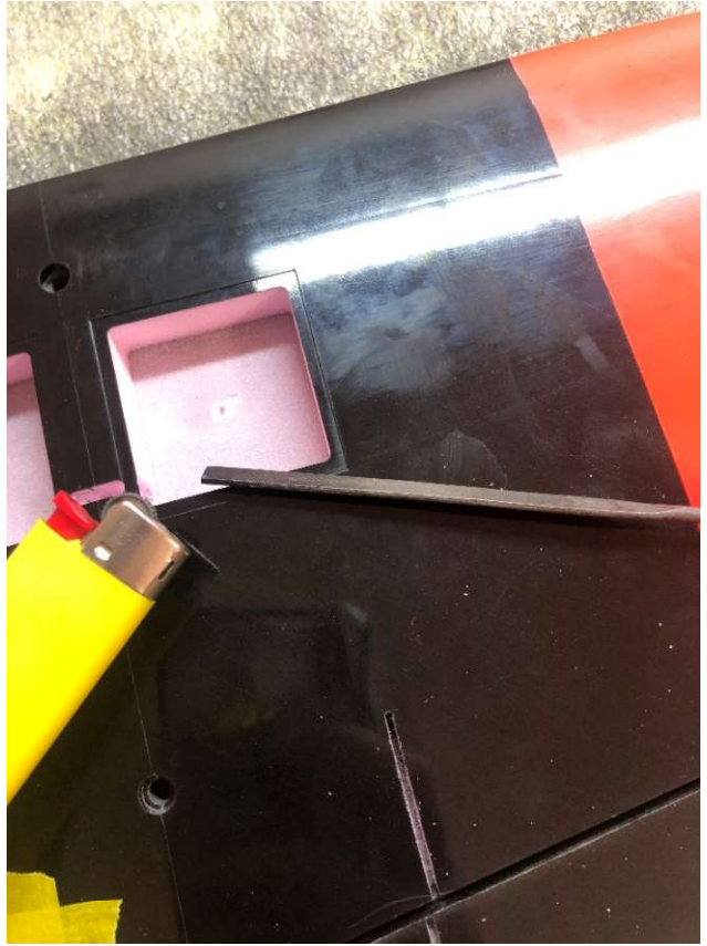
With a rectangular section jewellers file widen the slot in the foam to let the elevon linkage move freely.
