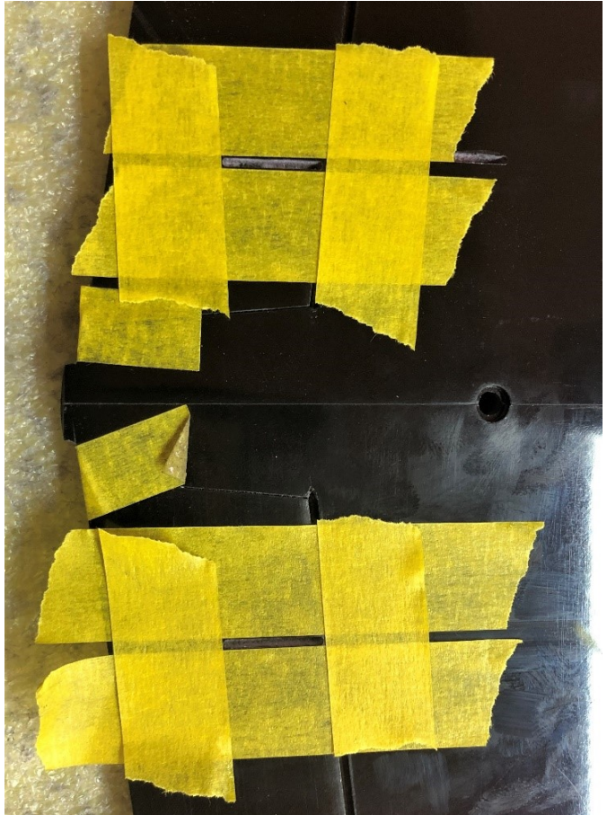
With a rectangular section jewellers file widen the slot in the foam to let the elevon linkage move freely.
