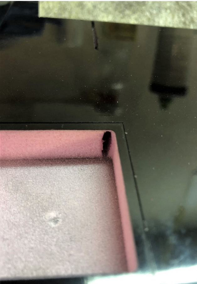
With a rectangular section jewellers file widen the slot in the foam to let the elevon linkage move freely.
