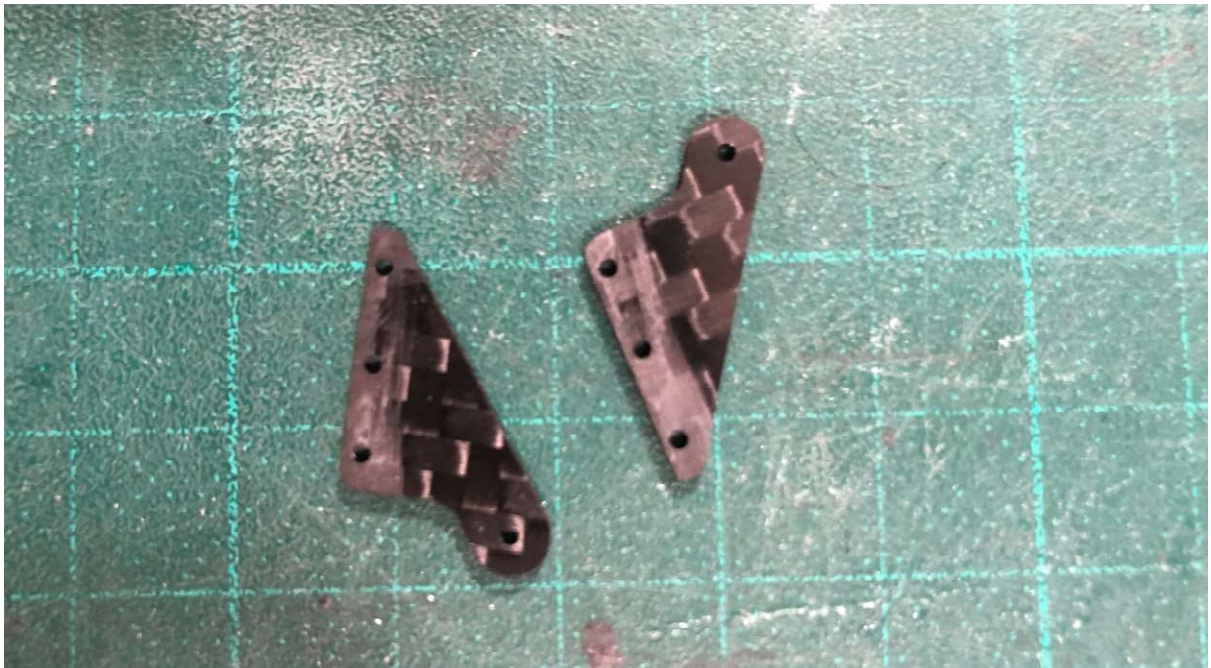
Roughen the base of the horns
